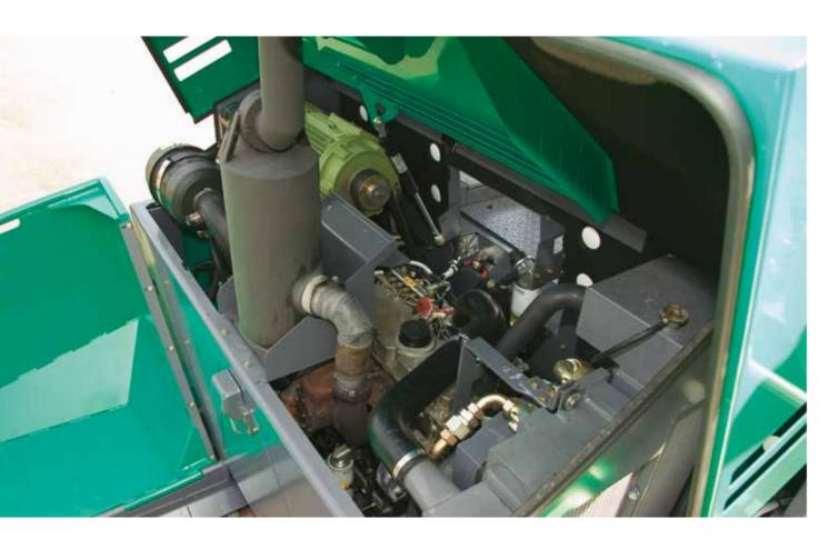
The SUPER 1800-2 is powered by a modern, liquid-cooled PERKINS engine rated at 129.6kW. The speed ranges MIN, ECO and MAX are available which select conveniently at the push of a button. ECO Mode is sufficient for 70 to 80% of all paving jobs. This mode reduces fuel consumption, wear and noise emissions.
