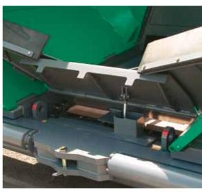
Like all VÖGELE pavers, supply of the SUPER 1800-2 with mix is a clean and safe process passing off swiftly. Thanks to a hydraulically operated hopper front (option), the mix inside the material hopper is directed right onto the conveyors and the entirety of mix properly conveyed in front of the screed.
