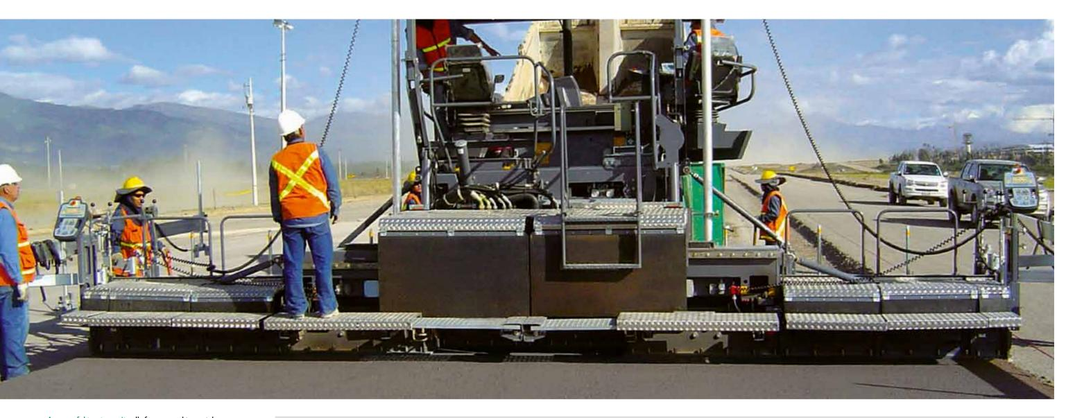
A powerful tractor unit calls for a screed to match. Each application has its particular requirements, so that in the end its up to the users' everyday tasks to decide which screed is the right one. For SUPER 1800-2, we offer a number of screed options and versions as far as equipment with compacting systems is concerned.
